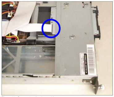
Figure 21: Connecting the data cable
